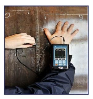
**The tiny ultrasonic flaw detector A1211 Mini** is a fully digital, small sized general purpose ultrasonic flaw detector. Provides an implementation of standard and specialized techniques of ultrasonic testing, performance, and accuracy.
