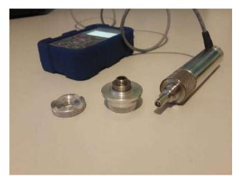
The device works with ultrasonic contact impedance (UCI) probe.
