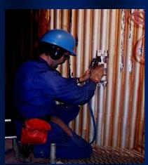
E-PIT<sup>™</sup> Tools are designed to inspect tubes & pipes from the outside surface to detect internal (ID) & external (OD) defects. This is useful for situations where a pipe must be inspected before it is taken out of service. E-PIT<sup>™</sup> can inspect through coatings (e.g. Yellow Jacket<sup>™</sup>) of up to 0.200" (5mm) thickness.
